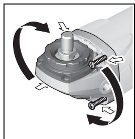
The machine head can be rotated with respect to the machine housing in 90° steps. In this manner, the On/Off switch can be brought into a more convenient position for special working situations, e. g., for cutting operations using the cutting guide with dust extraction protection guard 21 or for left-handed persons.
