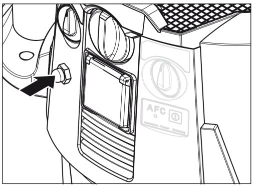
The fuse protects the socket against overload due to overcurrent. When it responds, a white pin becomes visible under the transparent cap. Pushing the pin will turn the power back on. Possibly the cause of the trip (e.g. the connected device) must be removed.
